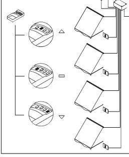
To OPEN using local command turns on the corresponding motor. To CLOSE using local command sends the motor down,
