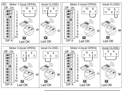
**B-3** This programme allows you to control all motors with 1x 2 button hand set. One button will open all the other button will close all. If you use one of the buttons during OPEN/CLOSING the doors will stop and wait for next command.
