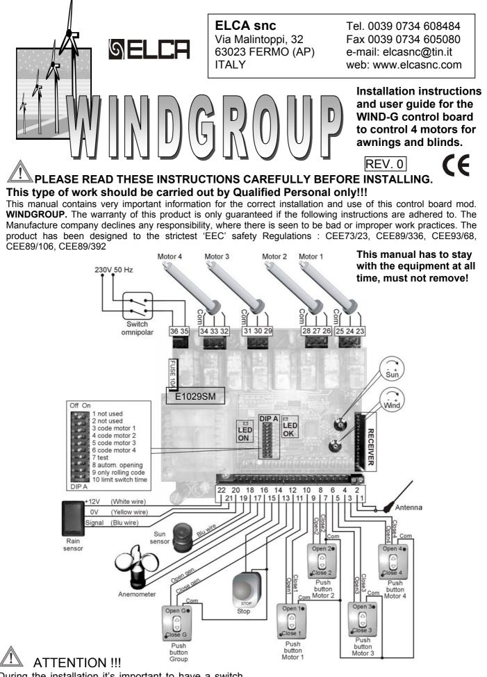
During the installation it's important to have a switch with contact opening of at least 3mm that ensures complete disconnection of the board and network. Please, ensure all motors are EARTHED in the proper manner.
